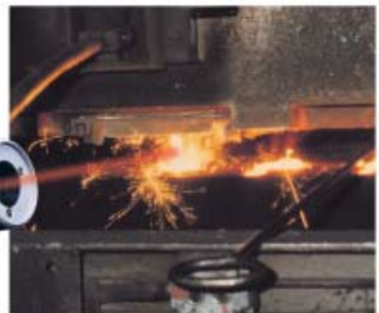
Temperature measurement of the pouring stream
