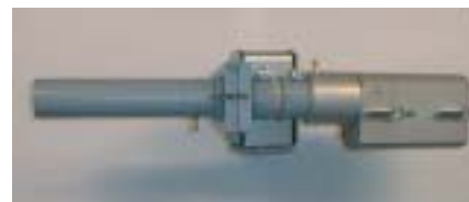
Assembly example with video camera consisting of cooling device, swivelling slope device, quartz disk hinge, axial play nozzle, protective pipe and dust screen.
