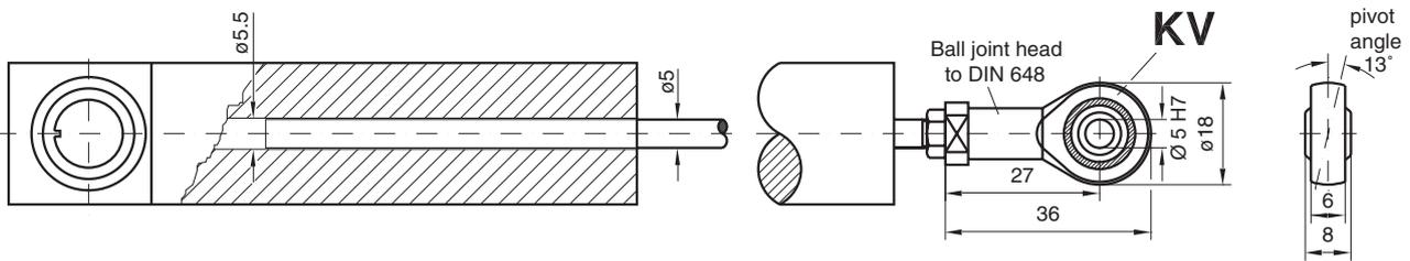
Version with ball joint on plunger (KFN) and on end of case (KHN), with rod guide, captivated
