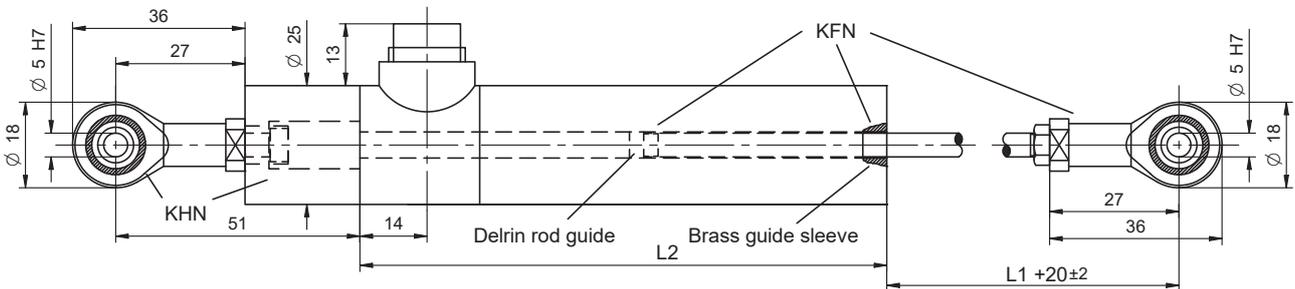
Gauge version (T) with return spring (up to 100 mm stroke),
