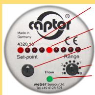
LED chain for display of flow speed
