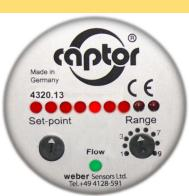
Measuring range adjusted to 3 m/s = 100% (9. LED)
